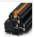
Double-level modular terminal block with suppressor diode as surge protection between both levels, disconnect knife in the upper level, nominal voltage: 24 V DC, for mounting on NS 32 or NS 35/7.5, closed housing, terminal width: 6.2 mm, terminal height: 68 mm
