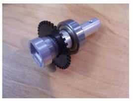
**Step 2:** Insert the axle assembly into the Bearing Block. This will be a very close tolerance fit. Take care to properly align the bearing with the block while maintaining a gentle pressure. Very gentle tapping with a wooden mallet can be used if required. This close-tolerance fit is by design.
