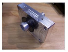
Step 3: Insert the motor shaft into the large diameter end of the drive axle.
