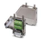
D-SUB connector, 9-pos. female connector, two cable entries <  $35^{\circ}$ , bus system: CAN, SUCONET K1, K2 (MOELLER), S-BUS (Saia), J-BUS (Merlin Gerin), pin assignment: 2, 3, 4, 5, 7, 9 to two screw connection terminal blocks
