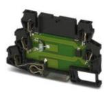
Double-level modular terminal block with two-stage surge protection for one two-wire impedance-sensitive signal circuit, separate ground connection, nominal voltage: 24 V DC.
