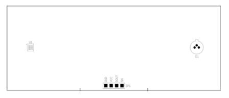
Referring to the back side of the LRF Module below, the Parallax Propeller (U2), its supporting electronics, and the camera interface circuitry are located on the right and the laser diode control circuitry is on the left. A dotted line (not printed on the actual LRF Module) indicates the recommended cutting point if the user wishes to separate the laser diode control circuitry from the rest of the LRF for custom modifications or projects.
