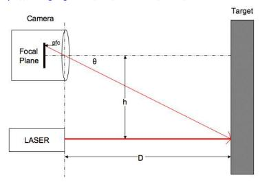
Referring to the figure, a laser diode module shines a laser spot onto the target object. The value h is a fixed, known distance between the center points of the laser diode and the camera (78 mm for the LRF Module). When the distance to the target object D changes, so do both the angle  $\theta$  and the value pfc (pixels from center), which is the number of pixels the centroid of the primary blob (laser spot) is away from the camera's center point.
