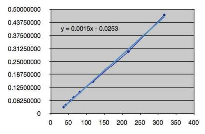
So, once the laser is shined onto the target object and the pfc value of the laser spot is received, an angle  $\theta$  can be calculated using the slope-intercept equation and passed to the trigonometric function to determine the actual distance the range finder is from the target object.
