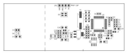
A Prop Clip (Parallax #32200) or Prop Plug (Parallax #32201) can attach to the four pads (JP2) on the back of the LRF for reprogramming of the Propeller's firmware.
