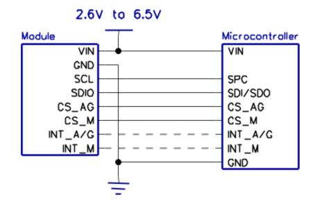
The accelerometer, gyroscope, and temperature sensor share a three-wire SPI interface, initiating communications by driving CS\_AG low, transmitting and receiving data on SDIO, clocking data on SCL, and ending communications by driving or letting CS\_AG float high. The magnetometer shares the SPI data and clock pins, but uses the CS\_M pin to start and end communications.
