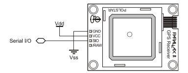
The on-board, four-pin header allows the GPS Receiver Module to be plugged into a solderless breadboard (on a Boe-Bot, for example). If the default "Smart Mode" is desired and the /RAW pin will be unused, the Module can be simply connected to its host with a standard three-pin servo extension cable.
