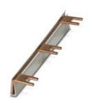
Wiring bridge with forked contact tabs for biconnect terminal blocks. Contact tabs with 17.5 mm pitch in arranged in irregular pitch steps. For wiring applications with lightning current and surge voltage arresters.
