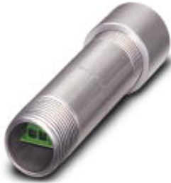
Screw on module for conduit systems, with two conductor protection for a 2-core floating signal circuit. Design: 24 V DC
