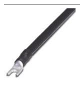
Wiring bridge flexible, diameter: 16 mm², with a fork-type cable lug on one side, length: 600 mm
