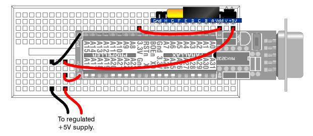
In this example, Vin is not connected. If the daughterboard requires it, an unregulated 6-9V supply could be connected to "V".
