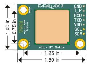
Pin spacing is standard 0.1" for a breadboard friendly design. Mounting holes are spaced by 1.25" and 0.75" center-to-center, with a .125" diameter, and accepts #4-40 screws.
