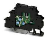
Modular terminal block with two-stage surge protection for a floating double conductor, separate PE connection, nominal voltage: 110 V AC, for mounting on NS 35/7.5, terminal block width 6.2 mm, terminal block height: 54.6 mm
