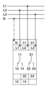
Correct phase connection: Output relay "R" picks up and yellow "REL" LED is  $\ensuremath{\mathsf{ON}}$
