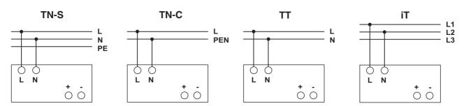
The 100...240 V AC connection is made using the L and N screw connections. The device can be connected to 1-phase AC networks or to two of the phase conductors of three-phase systems (TN, TT or IT networks in acc. with VDE 0100-300/IEC 60364-3) with nominal voltages of 100 V AC ... 240 V AC.
