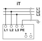
The connection for 3x 400 V AC ... 500 V AC is achieved using the L1, L2, L3 and PE screw connections. The device can be connected to 3-phase systems with nominal voltages 3x 400 V AC ... 500 V AC are connected. In the event of a phase failure, unrestricted operation is possible with nominal capacity. An operation in DC networks is also possible without any limitations.
