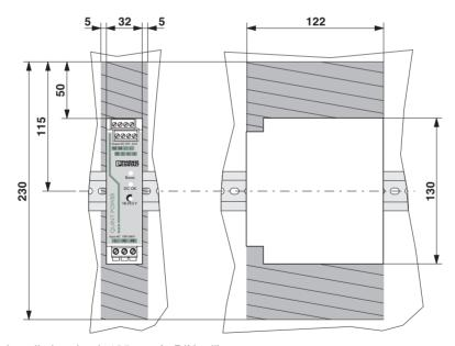
Slim-style installation: Installation depth 125 mm (+ DIN rail) (state at delivery)
