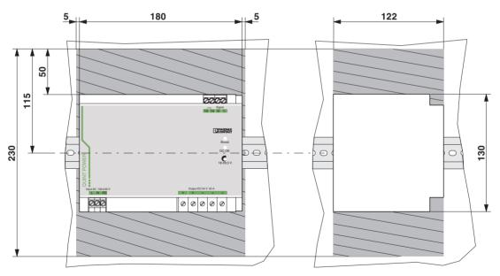
Slim-style installation: Installation depth 125 mm (+ DIN rail) (state at delivery)
