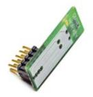
The HOPKEY contains information such as the transmission frequencies used and the hop sequence. This information is required e.g. when installing an additional receiver / repeater in an existing system.
