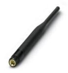
Omni-directional antenna, degree of protection IP55, 5 dBi gain, linear vertical, SMA (male), impedance 50 ohms, apex angle h/v 360°/45°
