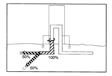
4.6 Several cables grounded at a common point present no problem for the Dyna-Coupler method. Even though signal is coupled into each cable, the cable with the Dyna-Coupler is clearly identifiable because it has the strongest signal.
