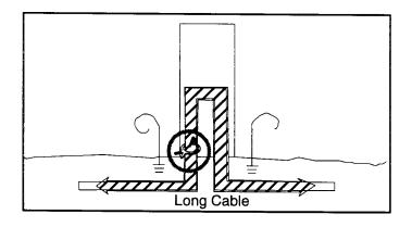
4.5 Clamping the Dyna-Coupler to a cable with drop lines or laterals puts full signal on the cable until the junction point. The signal may split evenly at the lateral as shown. When tracing, the speaker volume and signal level indication drops when the Receiver passes the junction. This is an easy way to find laterals.
