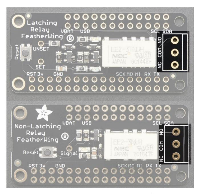
Both Wings have the same output, a 3-pin 3.5mm terminal block. The **COM** pin is what you should connect the signal you're planning to switch. If the relay is unset, the **NC** pin (Normally Connected) is mechanically connected to **COM**. **NO** (Normally Open) is mechanically disconnected.
