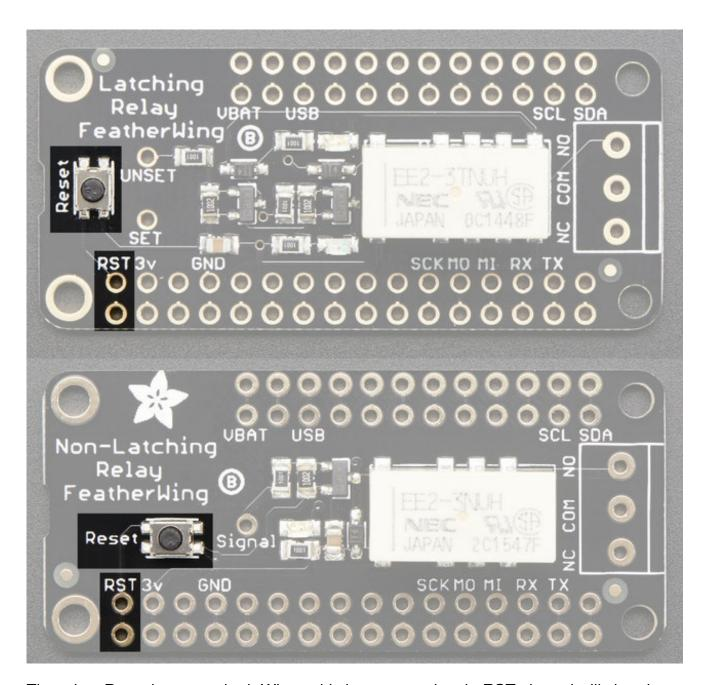
There is a Reset button on both Wings, this is connected to the **RST** pin and will short it to ground. It is not connected to the relay at all, its handy for restarting your Feather
