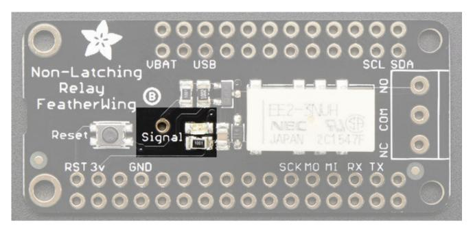
The **plain** relay uses a single pin for control. When the signal pin is floating or pulled low, the relay is 'open' or unset. When the signal pin is pulled high, the relay switches closed/set. A red LED next to the pin will let you know that the signal is high. You will need to solder a wire from this pin to whatever control pin you like using a wire
