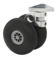
This kit contains a single, precision-machined caster assembly (two are required if you're mounting them to our Arlo Robot Base Kit - #28960). High-quality 6061 machined aluminum components (created in our machine shop in Rocklin, CA), are combined with smooth-rolling ball bearings and durable 3-inch Du-Bro pneumatic rubber tires. The dual independent tire design reduces vibration and drag, as well as increasing its load-carrying capacity.
