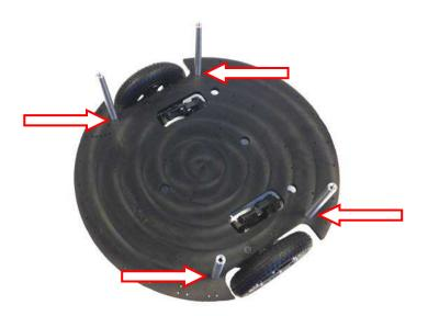
**Step 2**: Place the Top Deck onto the standoffs, making sure that the counter-sunk holes are face-up. Secure the deck with the four included  $\frac{1}{4}$  "- 20 x 5/8" flat-head screws.
