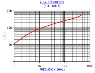
AGILENT E4991A Impedance/Material Analyzer HP 16092A-Test Fixture, REF #3399
