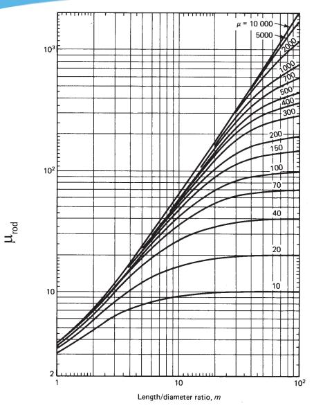
LI/AN $^2\mu_{rod}$  as a function of I /l. The results for a wide variety of ferrite rods are contained within the shaded area (dimensions in mm, L in H)
