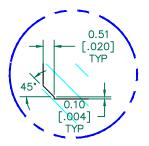
DETAIL "A" CHAMFER SCALE=6:1
