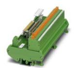
16-channel module for Honeywell C300 modules. The module is controlled by the control system via 37-pos. D-SUB or 50-pos. FLK. A screw connection (1+, 1-,...16+,16-) with knife disconnection is provided in the field. Module width: 170 mm
