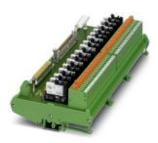
16-channel relay module for Honeywell C300 output modules. The module is controlled by the control system via 37-pos. D-SUB or 50-pos. FLK. A screw connection with knife disconnection is available in the field. Module width: 258 mm
