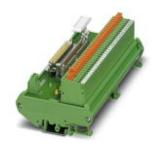
16-channel module with LED for Honeywell C300 modules. The module is controlled by the control system via 37-pos. D-SUB or 50-pos. FLK. A screw connection (1+, 1-,...16+,16-) with knife disconnection is provided in the field. Module width: 170 mm
