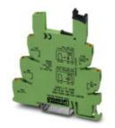
6.2 mm PLC basic terminal block for input functions with push-in connection, without relay or solid-state relay, for mounting on DIN rail NS 35/7,5, with sensor supply voltage distribution (BB), 1 N/O contact, input voltage 120 V AC/DC
