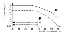
Derating curve for ELR H5-SC-24DC/500AC-9 100% operating time
