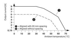
Derating curve for ELR H5-SC-230AC/500AC-9 100% operating time
