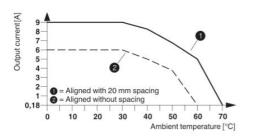
Derating curve for ELR H3-SC-230AC/500AC-9 100% operating time
