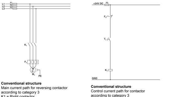
according to category 3 K1 = Right contactor F4 = Motor protection relay according to category 3 K1 = Right contactor T1 = Right, T3 = Reset F4 = Motor protection relay
