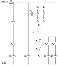
**Conventional structure** Control current path for contactor according to category 3 K1 + K2 = Emergency stop contactor K3 = Right contactor K4 = PSR SCP-24DC.../safety relay T1 = Right, T3 = Reset S2 = Emergency stop
