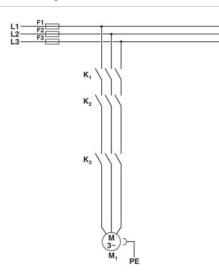
**Conventional structure** Main current path for contactor according to category 3 K1 + K2 = Emergency stop contactor K3 = Right contactor
