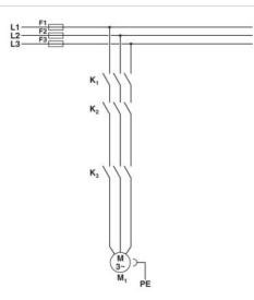
Conventional structure Main current path for contactor according to category 3 K1 + K2 = Emergency stop contactor K3 = Right contactor
