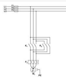
Conventional structure Main current path for contactor according to category 3 K1 = Left contactor K2 = Right contactor
