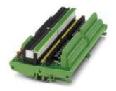
32-channel VARIOFACE relay module with screw connection and 50-pos. system connection. The power supply is designed redundantly, for Yokogawa ADV 151 card, module width: 232.5 mm
