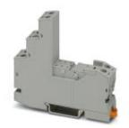
RIF-1... relay base, for miniature power relay with 1 or 2 changeover contacts or identical solid-state relays, screw connection, plug-in option for input/interference suppression modules, for mounting on NS 35/7,5
