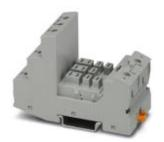
RIF-4... relay base, for high-power relay with 2 or 3 changeover contacts or 3 N/O contacts, screw connection, plug-in option for input/interference suppression modules, for mounting on NS 35/7,5
