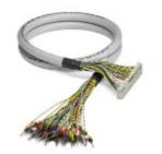
Round cable assembled with a 10-pos. socket strip and an open end. At the open end, the wires are labeled 1 to 10 and are fitted with ferrules, cable length: 1.5 m
