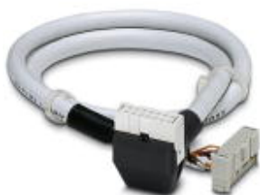
Round cable set for SIMATIC® TOP connect with 1 x IDC/FLK socket strip (16-position) on 1 x IDC/FLK socket strip (14-position), Cable length: 0.5 m
