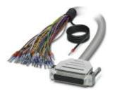
Assembled shielded round cable; connection 1: Single wires (25-position) (The wires are marked and fitted with ferrules. The braided shield is routed to a separate cable end.); connection 2: D-SUB socket strip (1x 25-position); cable length: 15 m
