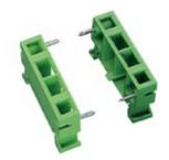
Side element with foot, labeling with SS-ZB, mounted along the length of the DIN rail NS 35/7.5. Height: 36 mm, width: 10 mm, length: 45 mm.
