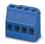
PCB terminal block, nominal current: 24 A, nom. voltage: 400 V, number of positions: 4, connection method: Screw connection with tension sleeve, mounting: Wave soldering, conductor/PCB connection direction: 0  $^{\circ}$
