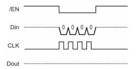
After reset, start a measurement by taking /EN low again, then shift-out %1000. Leave /EN low until checking the measurement status.
