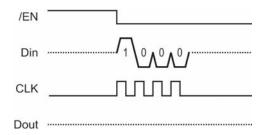
To check the measurement status, start by sending a positive pulse to /EN. Then, shift-out %1100, and shift-in the status flags. While the measurement is in progress, the end flag and error flag will both be 00. The compass Module may be polled for status repeatedly until the measurement is complete, at which point the end flag will change to 11. Upon receipt of %1100, discontinue polling. Leave /EN low, and move on to shifting-in the x and y-axis values.
