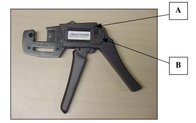
This tool incorporates an eccentric axle and an adjustment wheel to adjust and recalibrate to ensure correct crimp performance.
