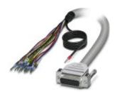
Assembled shielded round cable; connection 1: Single wires (15-position) (The wires are marked and fitted with ferrules. The braided shield is routed to a separate cable end.); connection 2: D-SUB socket strip (1x 15-position); cable length: 2 m
