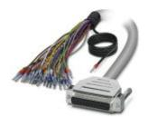
Assembled shielded round cable; connection 1: Single wires (25-position) (The wires are marked and fitted with ferrules. The braided shield is routed to a separate cable end.); connection 2: D-SUB socket strip (1x 25-position); cable length: 0.5 m
